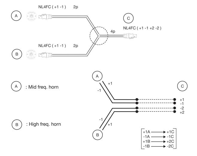
1) Cable between crossover and amp (not supplied): 2-pole cable (2.5 sq.mm minimum section per pole up to 15 m cable length, in addition we recommend switching to 4 sq.mm per pole), terminated with NI4Fc male connector (+1/-1 connected and corresponding to +1 red and -1 black on the amplifier, +2/-2 empty) to connect at the crossover input, which has NL4 female connector, standard or WP on request.
