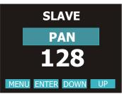
The SLAVE unit receives DMX signal from the MASTER unit. By setting all the SLAVE units connected to the MASTER, to DMX address 1, them will be synchronized with the Master unit following the chase selected on it, but running their own Pan&Tilt and Zoom position.
