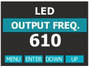
**OUTPUT FREQUENCY** Range = 610 Hz - 20 KHzDefault = 610 Hz
