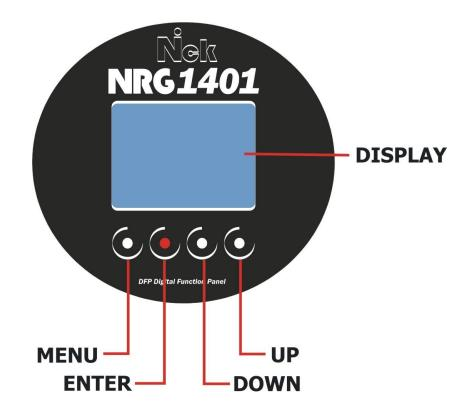
The NICK NRG 1401 display panel shows all the available functions. Using these functions, it is possible to change some of the parameters and add some functions. Changing the D.T.S. setting can vary the functions of the unit so that it does not respond to the DMX 512 used to control it. Carefully follow the instructions below before carrying out any variations or selections.
